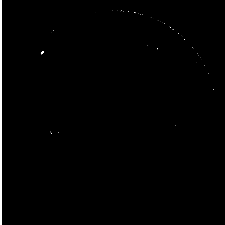
Figure 13. Initial result of thresholding with noise present throughout the image. A crescent of noise, seen in the upper right, has been misidentified as spots.
