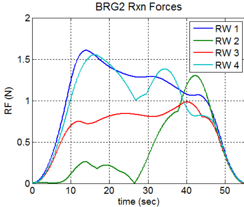
Figure 74. Bearing two reaction force magnitudes for an optimal slew, fixed-fixed configuration
