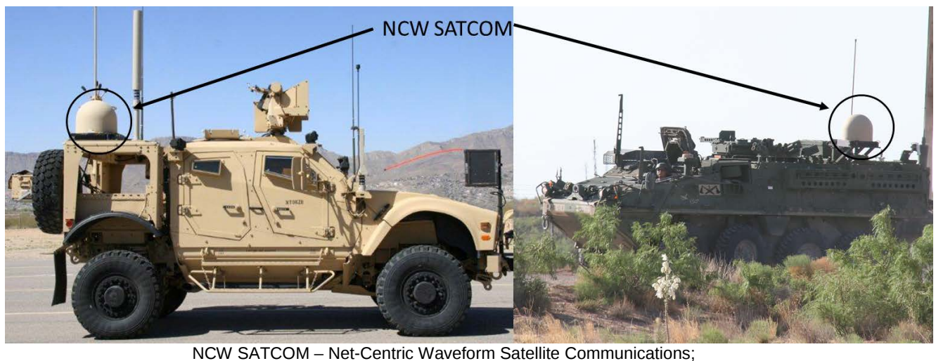
Figure 1-3. WIN-T Increment 2 SNE. Left: Integrated onto the MRAP. Right: Integrated onto the Stryker
