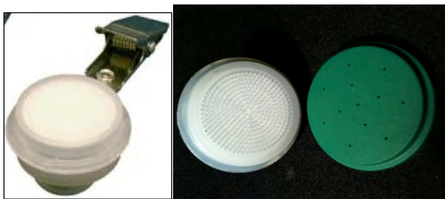
Figure 1a. SKC Ultra sampler with regular (white) and low-uptake cap (green).
