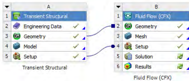
Figure 68. ANSYS Workbench, 2-Way FSI Connection.
