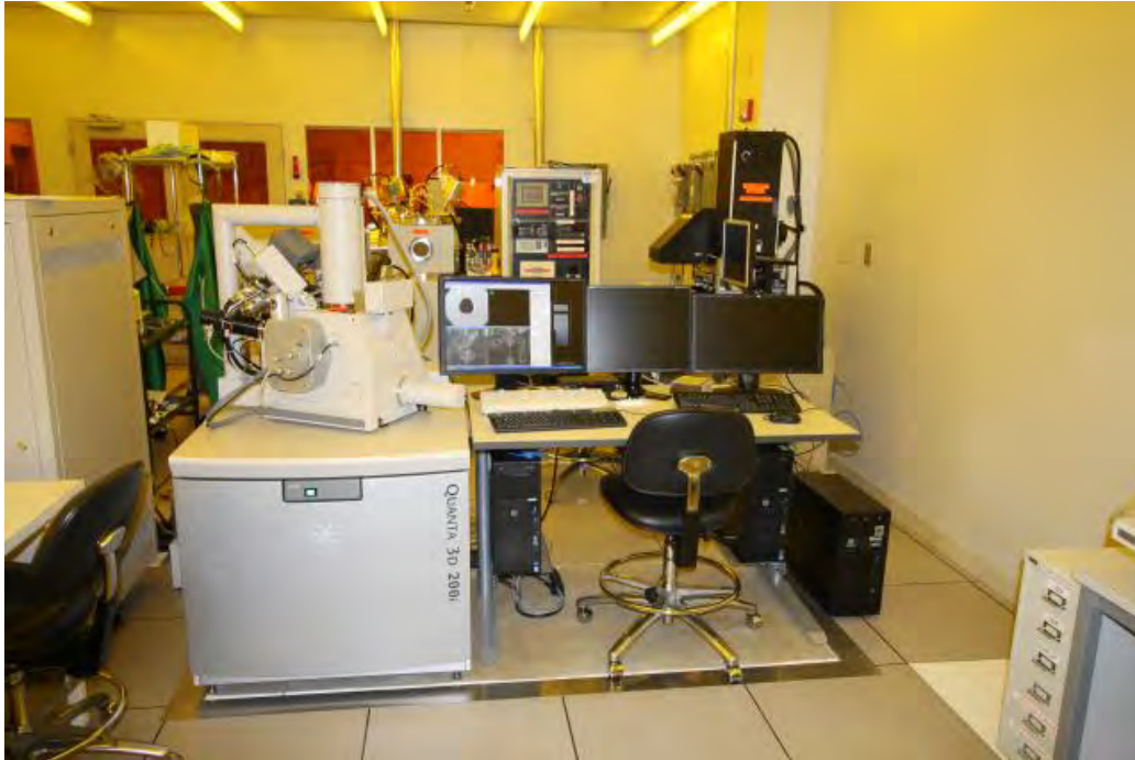
Figure C-7. Quanta 3D 200i scanning electron microscope used to provide SEM images of devices.
