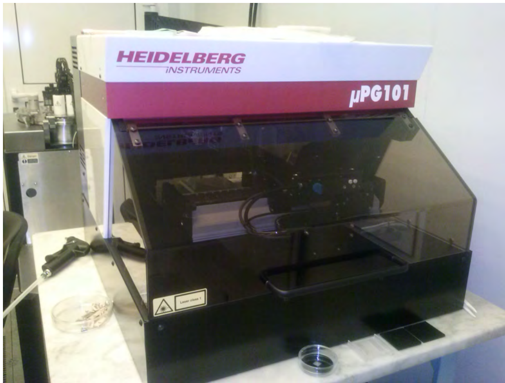
Figure C-2. Heidelberg \mu PG 101 direct write mask writer used for making 4" photomasks used during photolithography.
