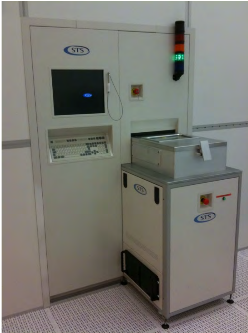
Figure C-4. STS Pegasus deep reactive ion etcher at the University of Michigan, Lurie Nanofabrication Facility.
