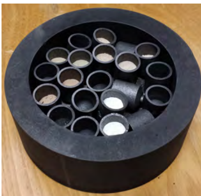
Figure 4.1: Loaded crucibles in graphite cup. Two replicates of each dusts were loaded for each test run. Empty crucibles were used to fill gaps between test samples to ensure samples remained upright during testing.
