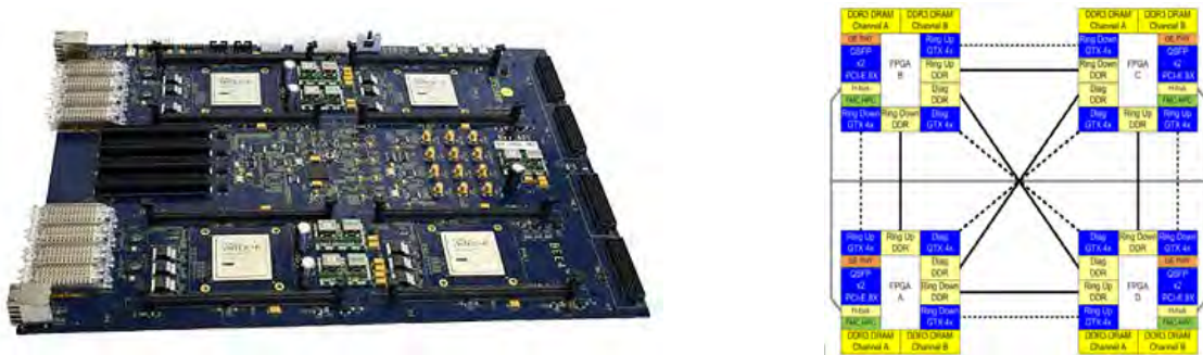
Figure 1: Interconnect Network Architecture of a BEE platform.
