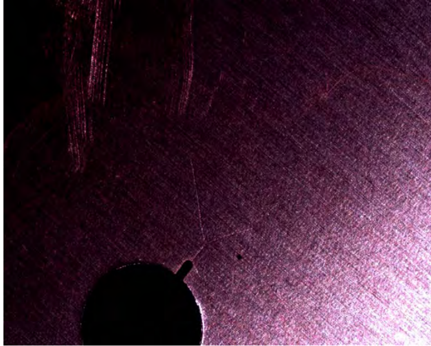
Figure B.5: Crack shape with 45^\circ of phase difference at 52,000 cycles in air environment.
