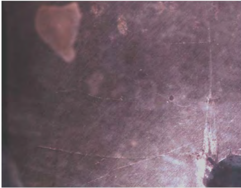
Figure B.21: Crack shape with 180^\circ of phase difference at 26,000 cycles in saltwater environment.
