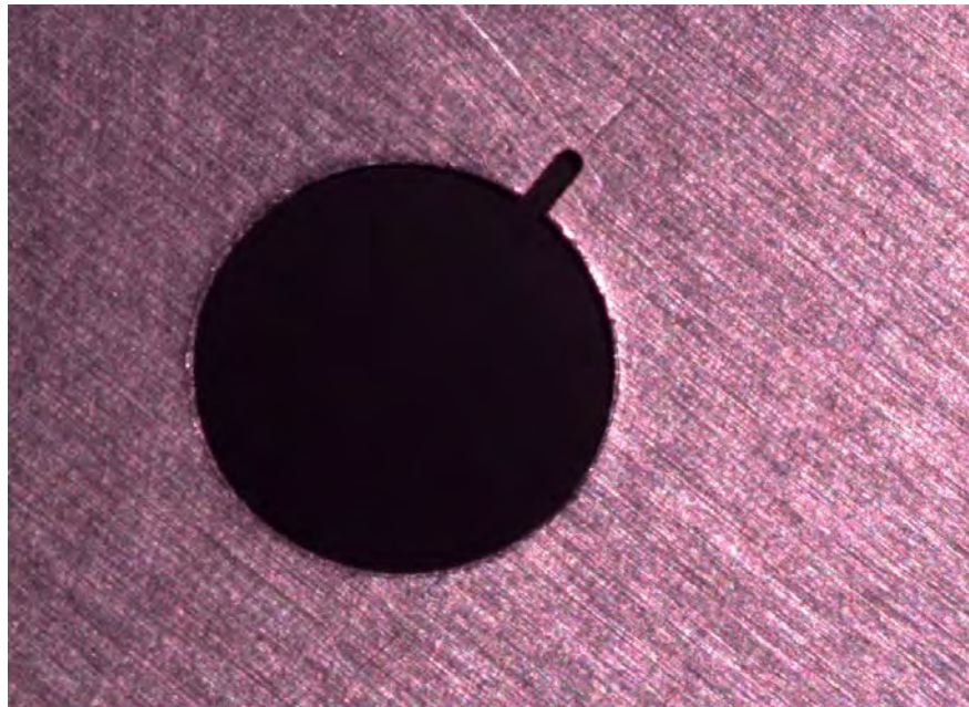
Figure B.4: Crack shape with 45^\circ of phase difference at the beginning of cycles in air environment.
