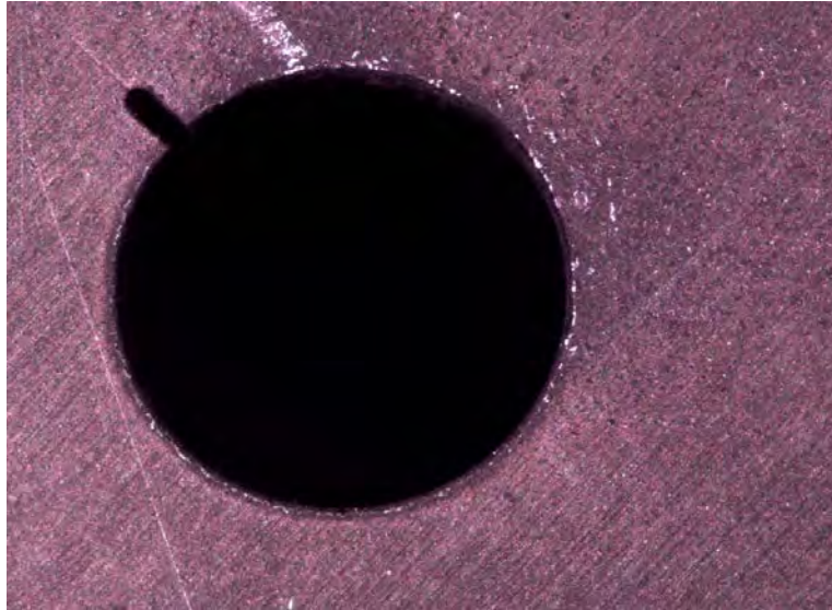
Figure B.1: Crack shape with 45° of phase difference at the beginning of cycles in air environment.
