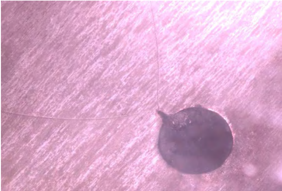
Figure B.15: Crack shape with 90^\circ of phase difference at 174,500 cycles in air environment.
