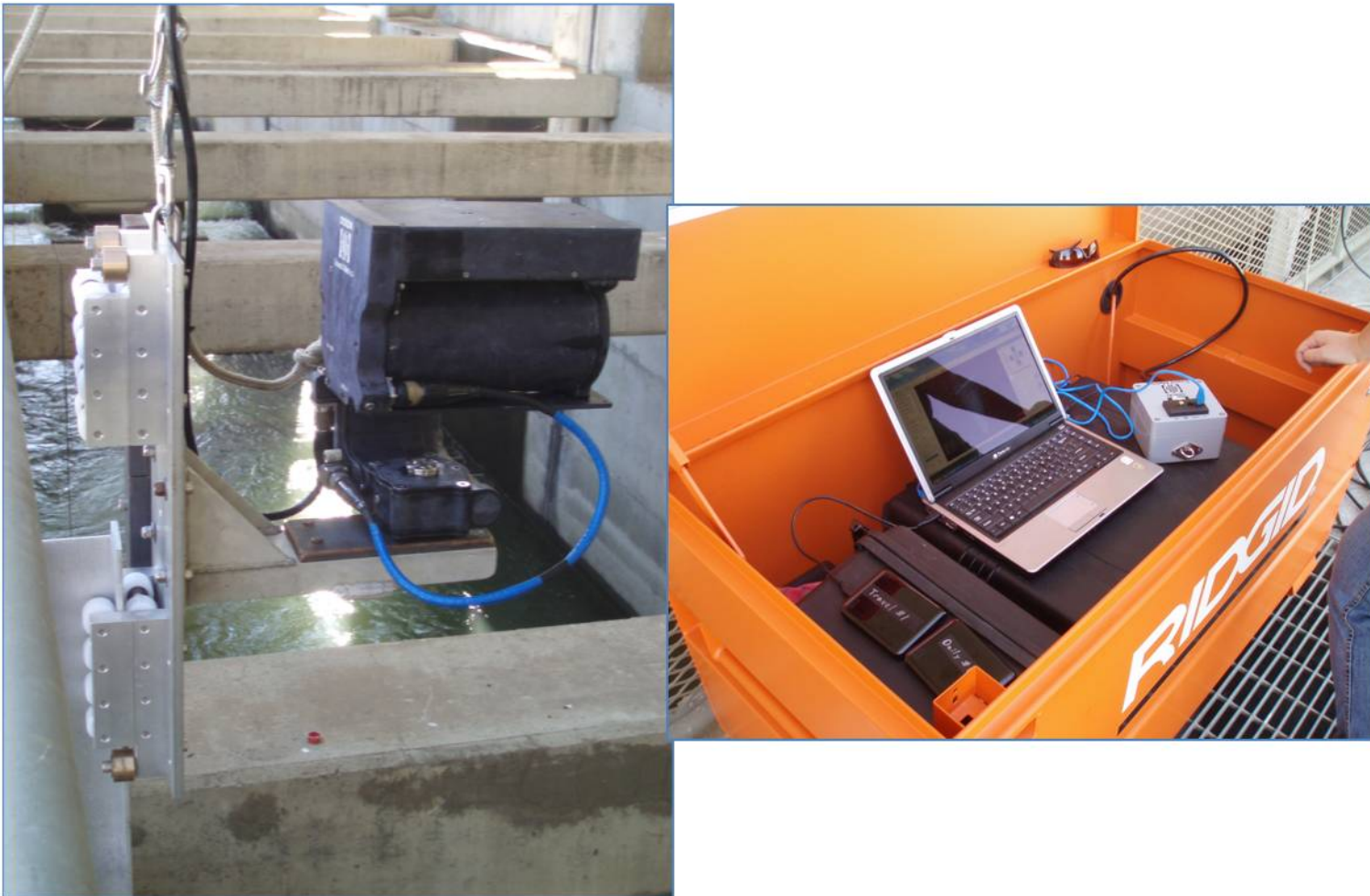
Figure B7. A) DIDSON camera mounted to the aluminum trolley at John Day I-beam number 4 (JD4) and B) the topside control system and setup housed in a protective metal workbox.
