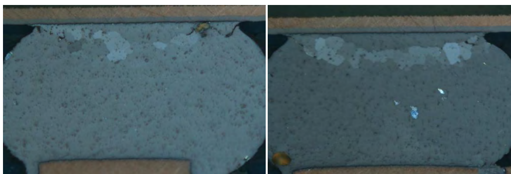
Figure 3.26: Cross polarizer images of SAC305 solder joint cross sections after 971 thermal cycles from 25°C to 100°C.
