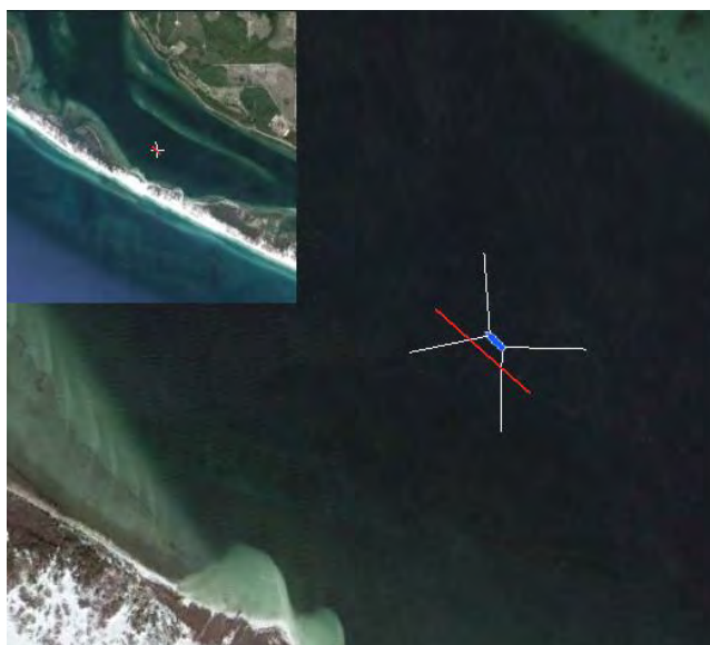
Figure 27: Configuration of the R/V Sharp and mooring lines relative to the MBES track The inset shows the mooring location relative to the shoreline along the bay.
