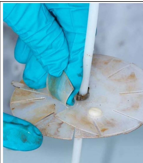
Figure 44. In well flow inhibitor used by ProHydro, Inc. to limit vertical solute migration in a well.
