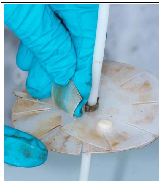
Figure 13. In well flow inhibitor used by ProHydro, Inc. to limit vertical solute migration in a well.
