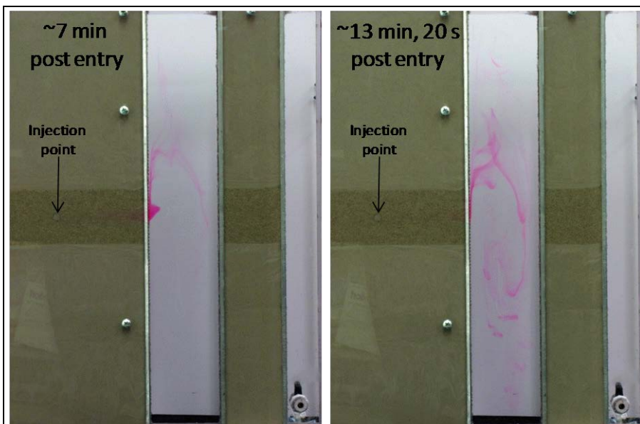
Figure 45. Results of a dye tracer experiment conducted at INL investigating transport to a well of a negatively buoyant injection solution. The upward movement of the dye upon entry into the well is hypothesized to reflect thermal convection due to inadvertent warming of the injection solution.
