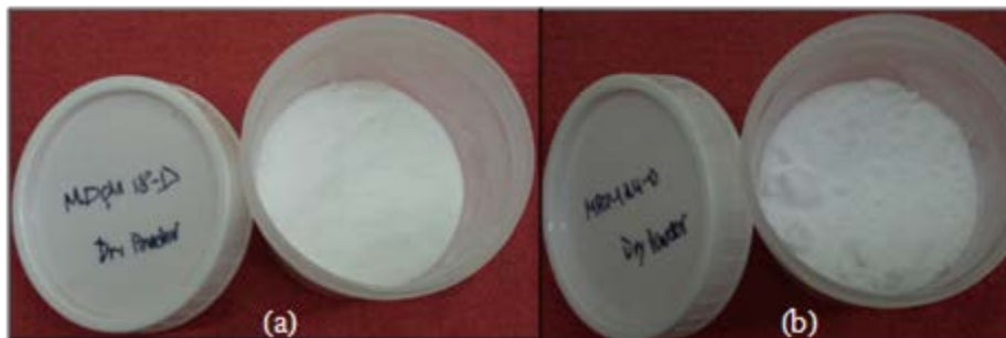
Figure 2-3. Micro-encapsulated PCM materials: (a) Microtek 18D sample, and (b) Microtek 24D sample.
