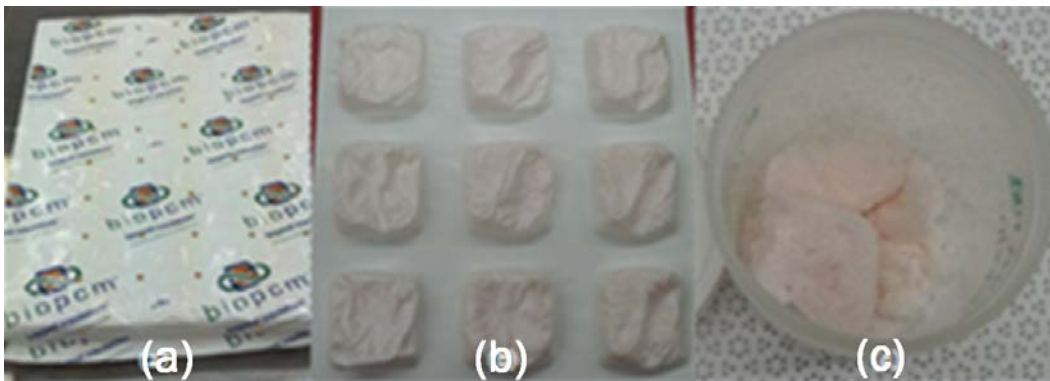
Figure 2-1. BioPCMat™ materials: (a) blanket with pouches of mixture of palm oil and soy oil, (b) sample put into the environmental chamber for testing, and (c) the appearance of BioPCM sample (extracted from one pouch).
