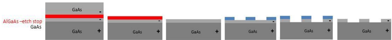
Figure 7. Steps in the GaAs wafer bonding process—the presence of an etch stop layer secures the uniformity of the inverted layer, but still requires a MBE reactor.
