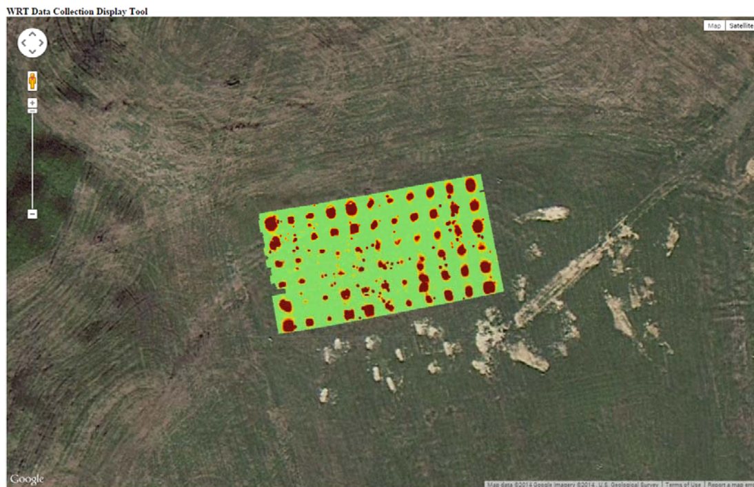
Figure 21. OPTEMA data map (400 – 500 microsecond time gate sum of Transmit Z-/Receive Z- channels) of the calibration grid.
