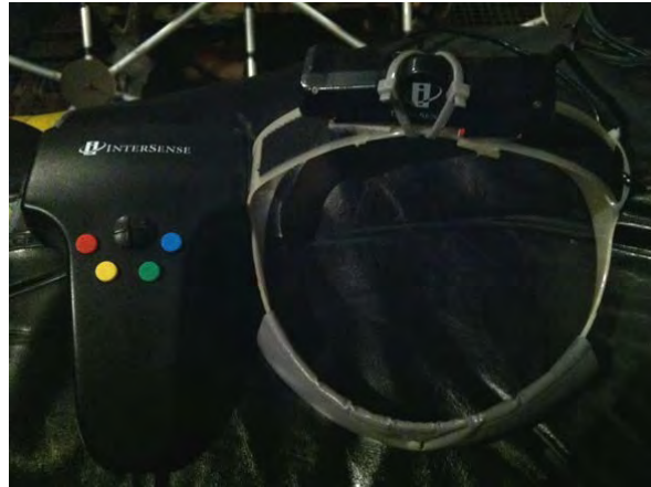
Figure 29. Intersense IS-900 tracking system
