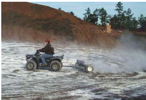
Using an all-terrain vehicle and a drop spreader to apply lime to soil surface at a HGR (Larson et al., 2007).
