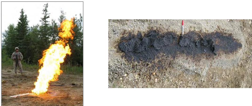
Figure 5-5. Example of burning excess propellant on the ground (left). Propellant residue remaining after burn is completed (right). Photographs provided courtesy of Michael R. Walsh, U.S. Army Cold Regions Research and Engineering Laboratory, Hanover, N.H.
