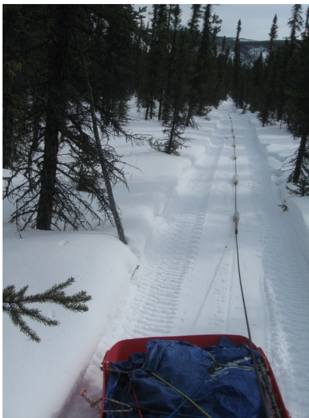
Figure 16. The OhmMapper system pulled by a snowmobile on a packed trail.
