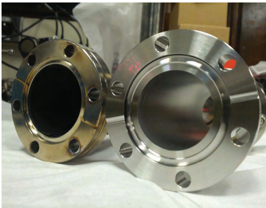
Figure G.1: 2.75" conflat nipple with an OFHC copper insert coated with copper(II) oxide (left) and bare (right).
