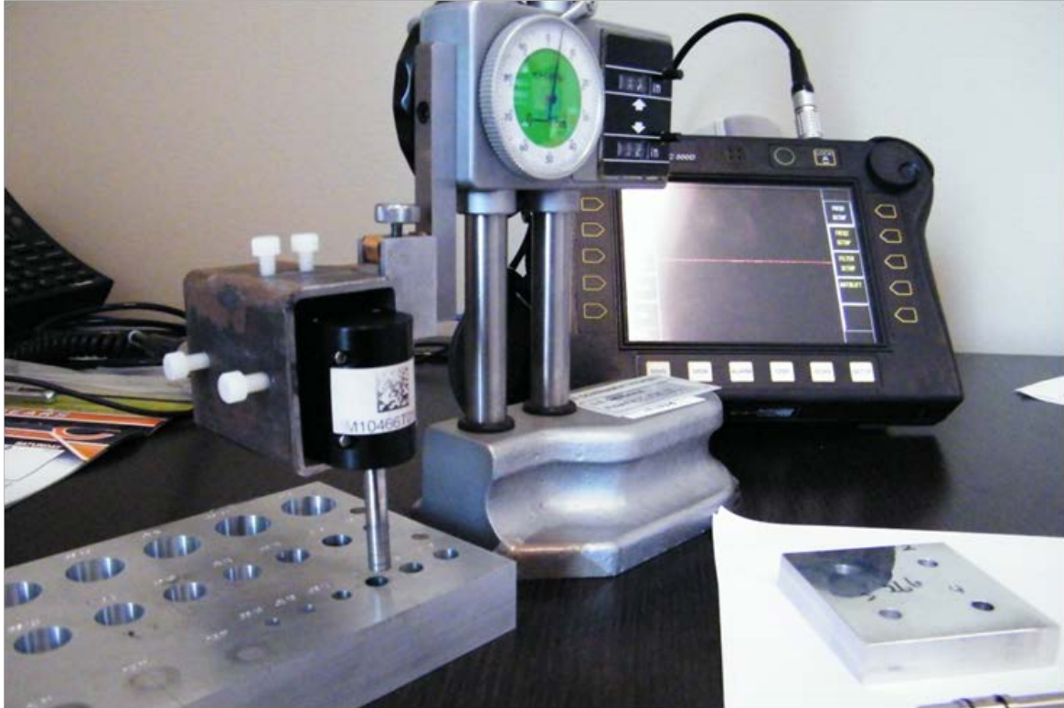
Figure 69. Equipment for the ET – Bolt Hole inspection of cold worked holes specimens.
