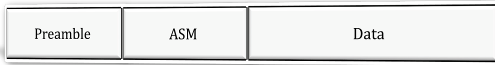
Fig. 1: INET Packet structure
