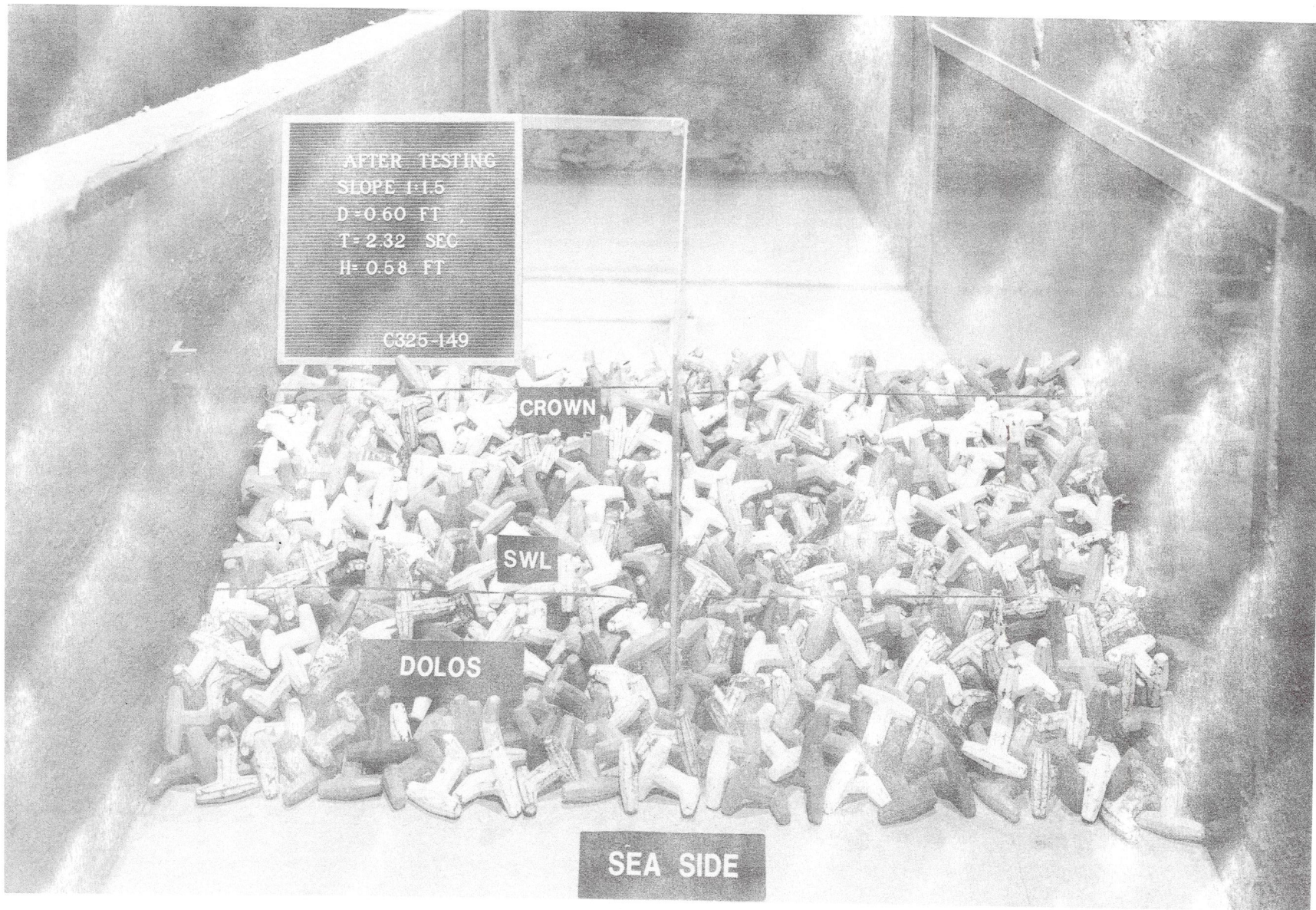
Photo 7. Sea-side view after attack of 2.32-sec, 0.58-ft waves; d = 0.60 ft; W_a = 0.589 lb; 1V-on-1.5H-structure slope
