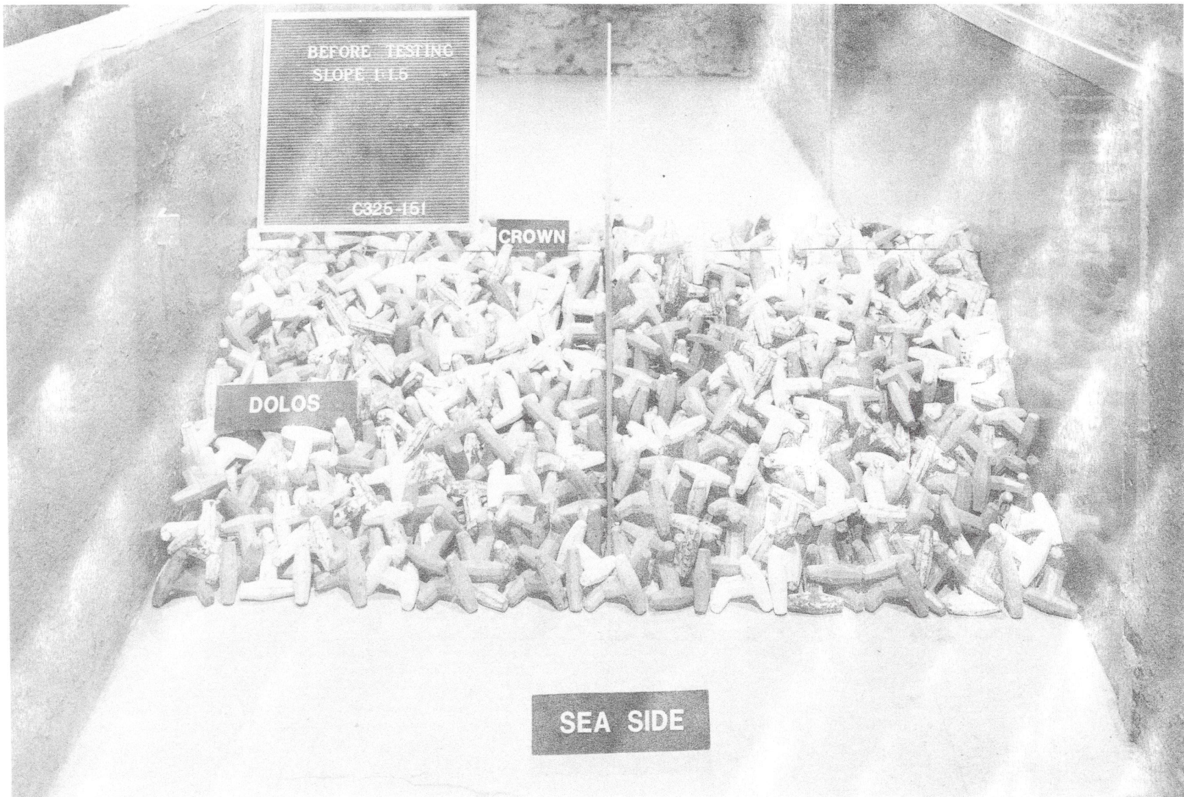
Photo 2. Sea-side view of a typical test section before wave attack at a 1V-on-1.5H-sea-side-structure slope; W_a = 0.589 \text{ lb}
