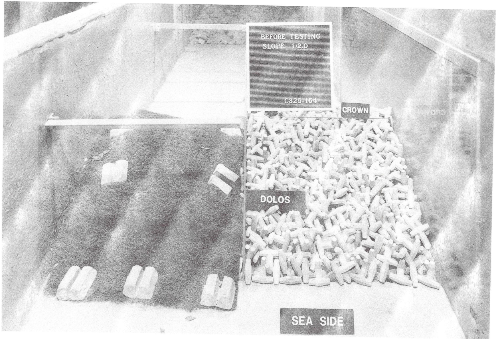
Photo 4. Sea-side view of a typical test section before wave attack at a 1V-on-2H-sea-side-structure slope; W_a = 0.442 \text{ lb}
