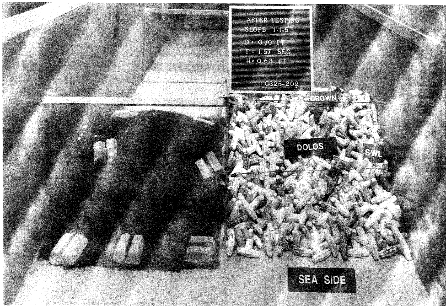
Photo 6. Sea-side view after attack of 1.57-sec, 0.63-ft waves; d = 0.70 ft; W_a = 0.589 lb; 1V-on-1.5H structure slope
