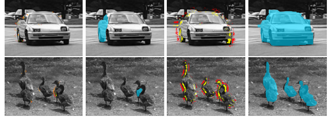
Figure 5: Occlusion cues from the current frame alone ( O_t ), with occluded points ( \Omega ) in red and occluder points ( \bar{\Omega} ) in yellow, (column 1) fail to segment the objects (column 2). However, aggregating constraints over time ( \bar{O}_t ) (column 3) successfully recovers all of them (last column).
