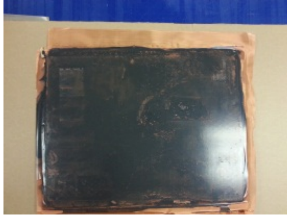
Figure 38: Sample with Copper Mesh Adhered to Both Surfaces
