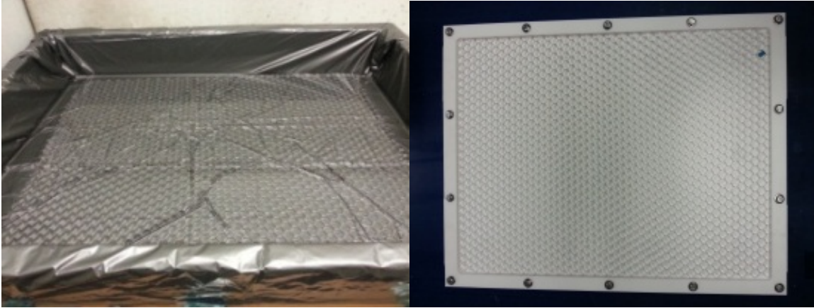
Figure 34: Nitric Acid Etching of Aluminum Honeycomb
