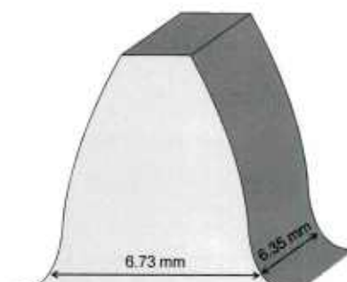
Figure 15: NASA-designed spur gears
