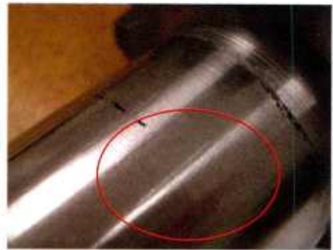
Figure 13. Stainless Steel Thermal Spray Shaft Denting
