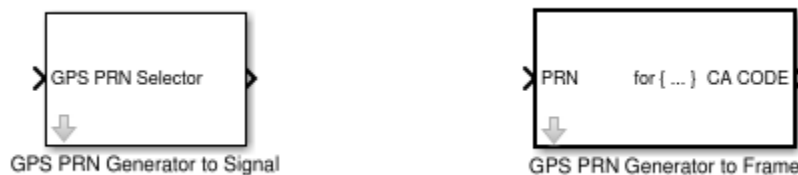
Figure 5 from left to right, the two different flavors of the C/A Code generator
