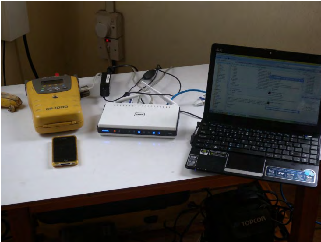
Figure 2 – System installed at one of the SEGAL stations (Rodrigues, Mauritius), which data are now accessible to SCINDA since the installation of the router (in the center).
