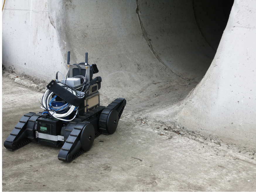
Figure 39. AVATAR ® II robot equipped with sensors and radios about to enter a storm drain near the international border south of San Diego.
