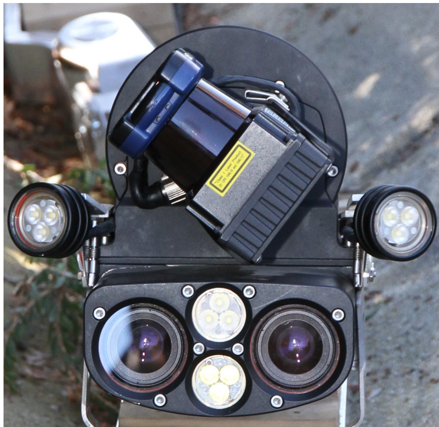
Figure 13. NREC MultiSense-SL perception sensor includes a rotating lidar, stereo cameras, and strobing LED lights.
