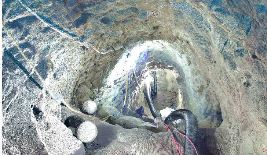
Figure 45. Point cloud of steps leading down into the tunnel, collected by the Focus3D sensor. Two of the spherical fiducials used to stitch scans together can be seen on the left.
