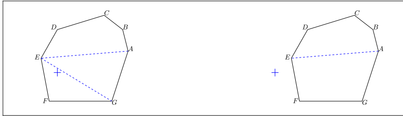
Fig. 4 Two example Mdiff sets demonstrating how GJK operates. The set on the left includes the origin while the set on the right does not (the origins are indicated by the small plus signs). The dashed lines indicate the segments added to the simplex by GJK.
