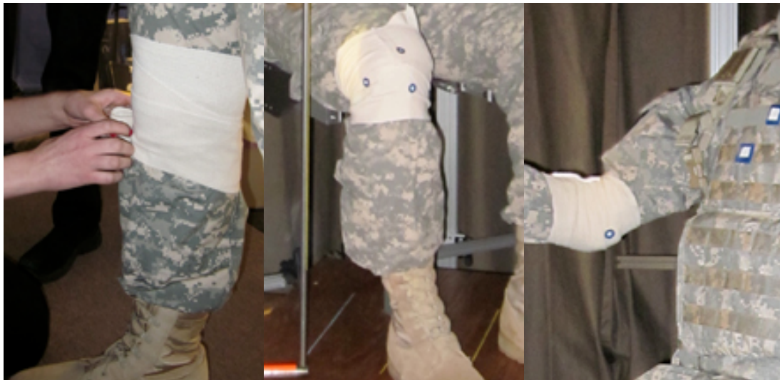
Figure 23. Right knee and elbow wrapped with an elastic bandage while the soldier was standing. Each time the soldier changed posture, Velcro targets were centered on the landmarks.
