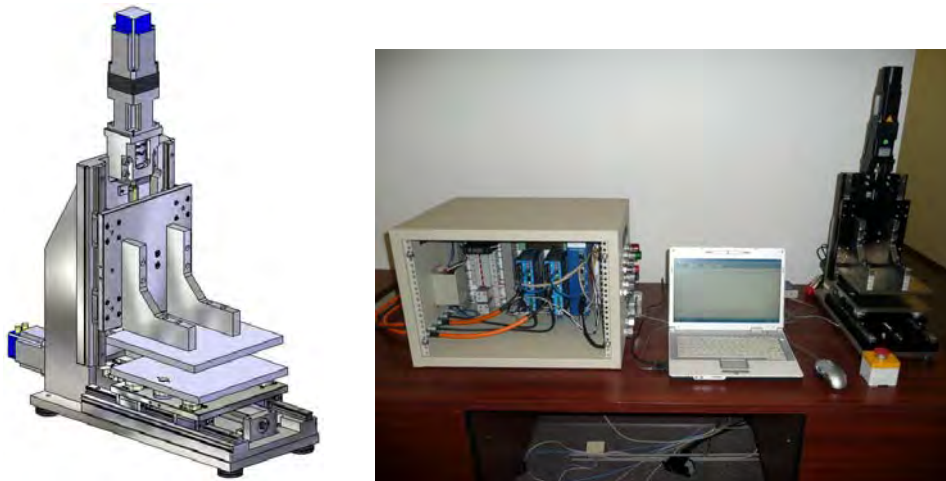
Figure 2.7. The designed CNT shear pressing device (left) and the actual computer-controlled shear press built by 3TEX, Inc. (right).
