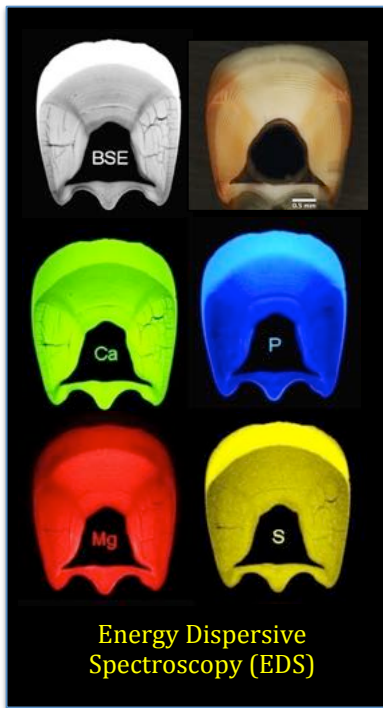
Figure 6. Elemental analysis of cross-section of dactyl club via EDS. Back-scatter electron micrograph highlighting mineral rich impact region (upper, left); optical micrograph (upper, right); Calcium map (middle, left); Phosphorus map (middle, right); Magnesium map (lower, left); Sulfur map (lower, right).
