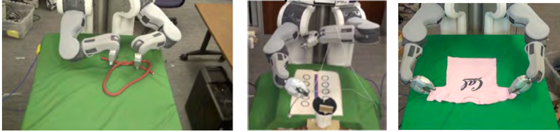
Figure 1: Autonomous knot-tying, suturing, and folding of a t-shirt. Key insight in this project was how to build on existing techniques for non-rigid registration to enable generalization of motions by warping them appropriately from training scene to test scene.
