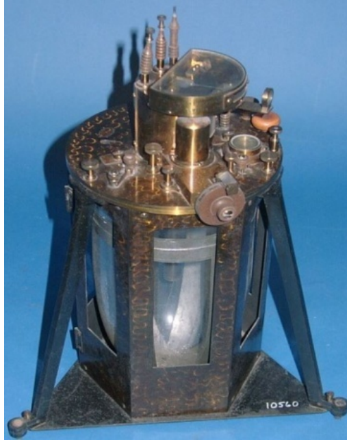
Figure 163: Sir William Thomson's Quadrant Electrometer [87]
