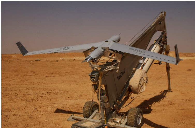
Figure 1.1. Scan Eagle aircraft on launcher in Iraq [28].
