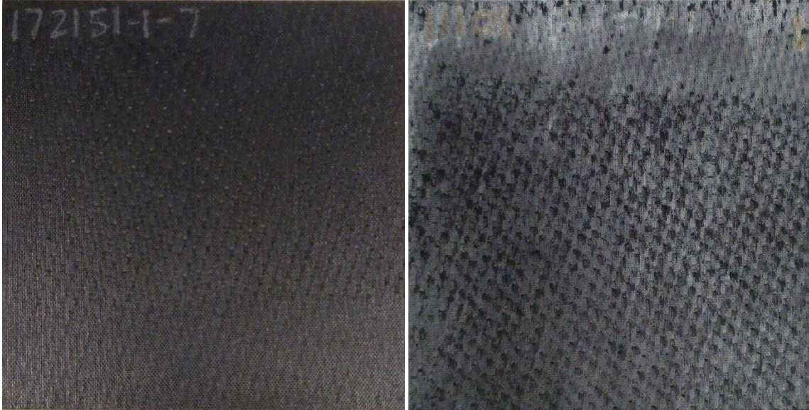
Figure B.1: Hi-Nicalon™/SiNC – Virgin plate 11107 (left); 10h 1300°C exposure plate 11101 (right). Exposed plate exhibits discoloration.
