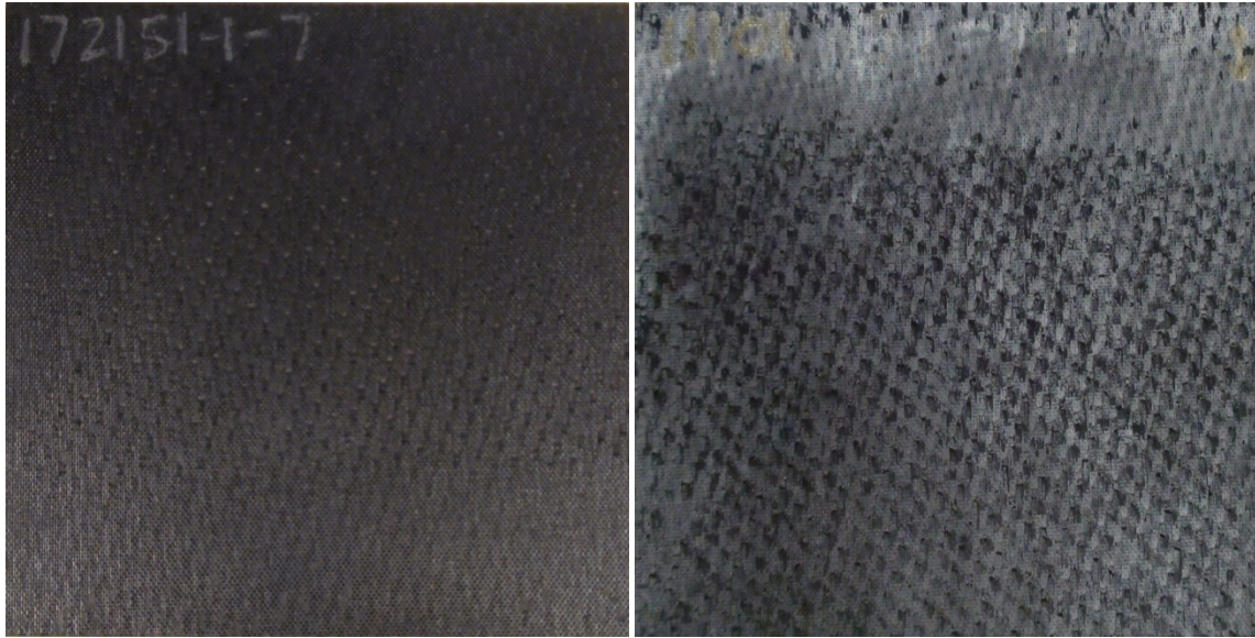
Figure 11: Example of Hi-Nicalon™/SiNC plate discoloration due to heat treatment – virgin plate (left); exposed plate (right).
