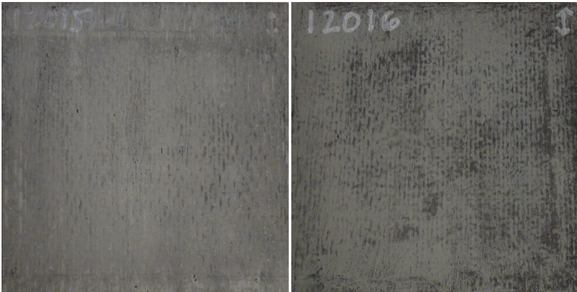
Figure B.6: HexTow ® IM7/SiC – 100h 1300°C exposure plate 12015 (left); 100h 1200°C exposure plate 12016 (right). Exposed plates exhibit discoloration.
