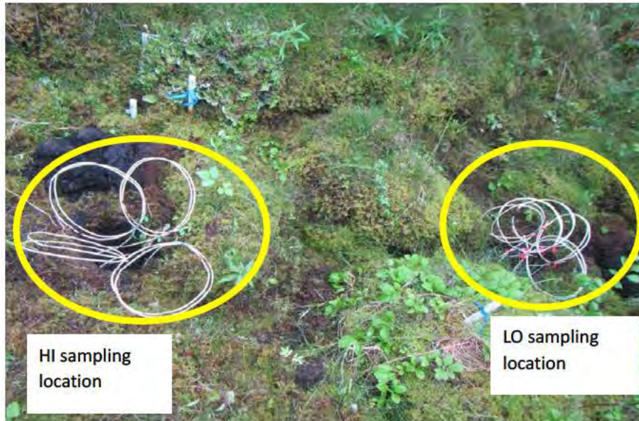
Figure 4. An example of an oxidation-reduction potential sample scheme displaying replicate Pt electrodes. Note that adjacent HI and LO sample locations are within 1 m of each other.
