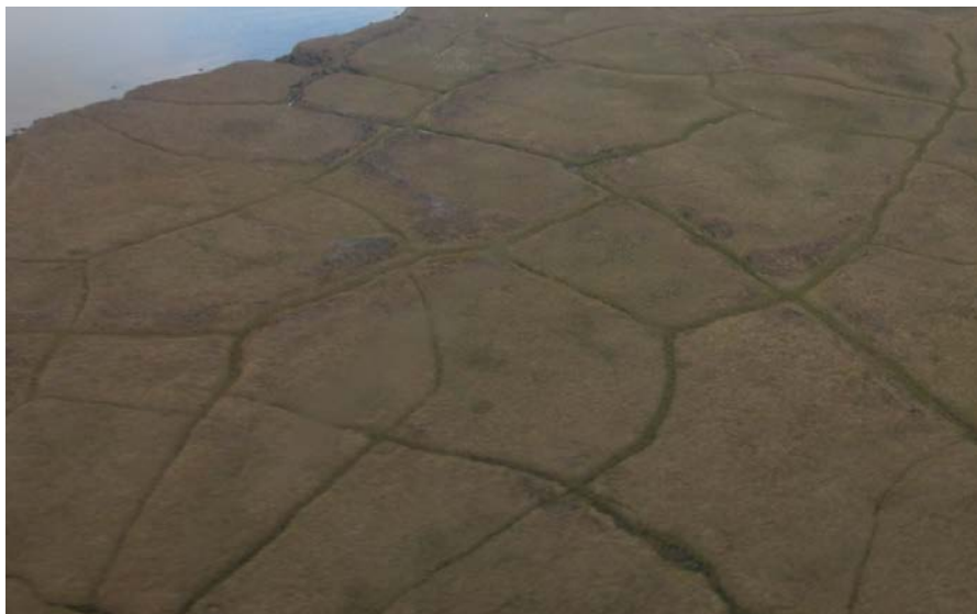
Figure 2. Ice wedge polygons along the Arctic Ocean Coast near Barrow, AK. The low-lying linear features are underlain by ice wedges; and the regions in between, also permafrost, are composed of frozen gravels, sands, and silts with an ice-rich matrix.
