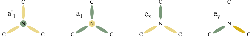
Figure 2.1: Single electron orbitals of the NV center. The nitrogen and three carbons surrounding the vacancy are shown, and the perspective is along the NV axis. The color scale roughly represents the sign and occupation of each orbital.
