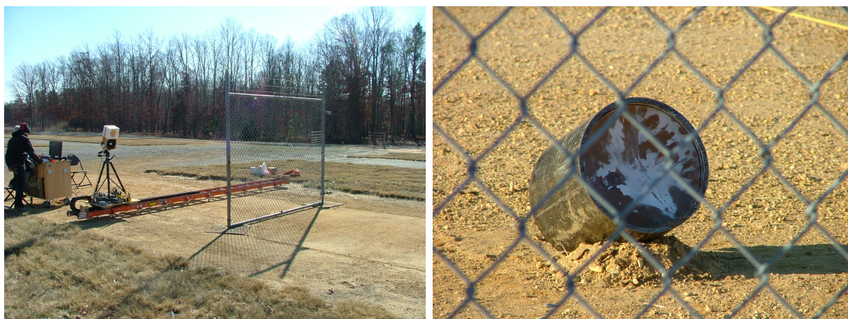
Figure 4.1: (left) The concave capped cylinder is shown behind the chain link propped so that copper shell is directed toward the scanner. (right) A section of chain link fence in place in the scanner range. Note that the target was not in place for the photo.
