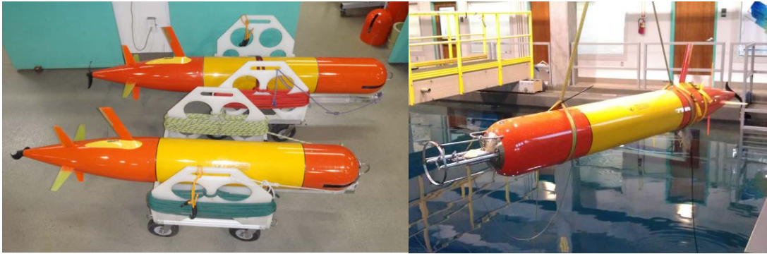
Figure 2: (left) Two Tethys-class long range AUVs. Tethys is in the foreground with the standard short nose configuration, and Daphne is in the background with a longer nose for increased payload volume. (right) Daphne with a turbulence sensor package, prior to deployment.
