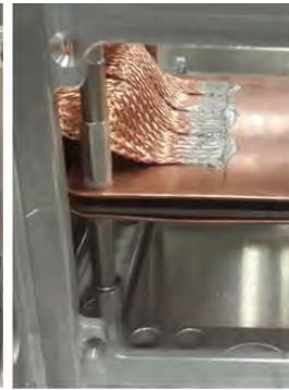
(b) Two Views of Soldered Copper Braids Used in ET-H
