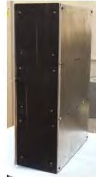
(c) The CubeSat with Black Tape Covered 3U Size Radiator, ET-J
