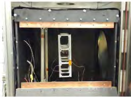
(c) The Chassis inside TVAC
