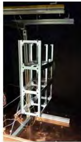
(b) The Chassis including Heaters in TVAC
