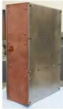
(b) The CubeSat with 3U Size Radiator, ET-I
