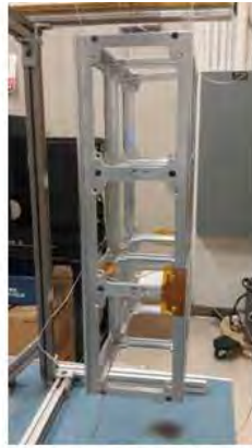
(a) The Chassis, Hung from the Test Stand
