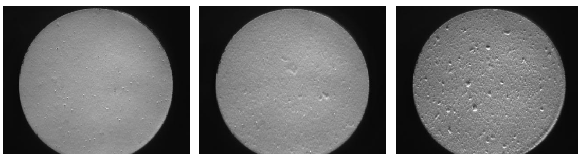
Figure 9 Schlieren images for pure \text{Y}_2\text{O}_3 , 1%Er: \text{Y}_2\text{O}_3 and 5%Er: \text{Y}_2\text{O}_3 ceramics (from left to right).
