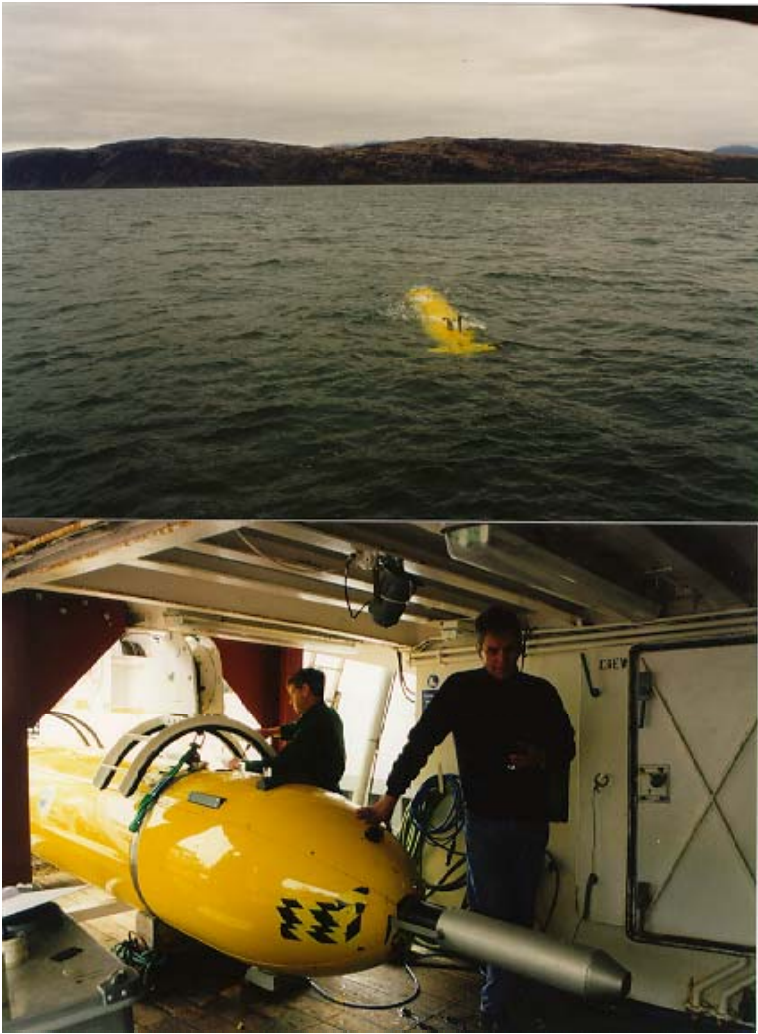
Figure 1. Top panel is AUTOSUB underway for near surface test in Loch Linnhe Scotland. The lower panel shows the turbulence pressure case covered with the retractable sheath that protects the delicate probes when the vehicle is on the surface.
