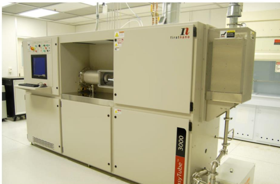
Figure 2: EasyTube3000 CVD System used for annealing and graphene growth
