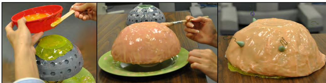
Figure 6. Pouring of silicones and first HFP
