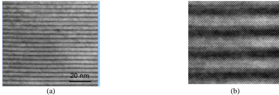
Figure 13. (a) TEM and (b) HRTEM images of MWIR T2SL grown on GaSb substrate with optimized growth conditions [Images by courtesy of Dr. S. J. Lee, KRIS]
