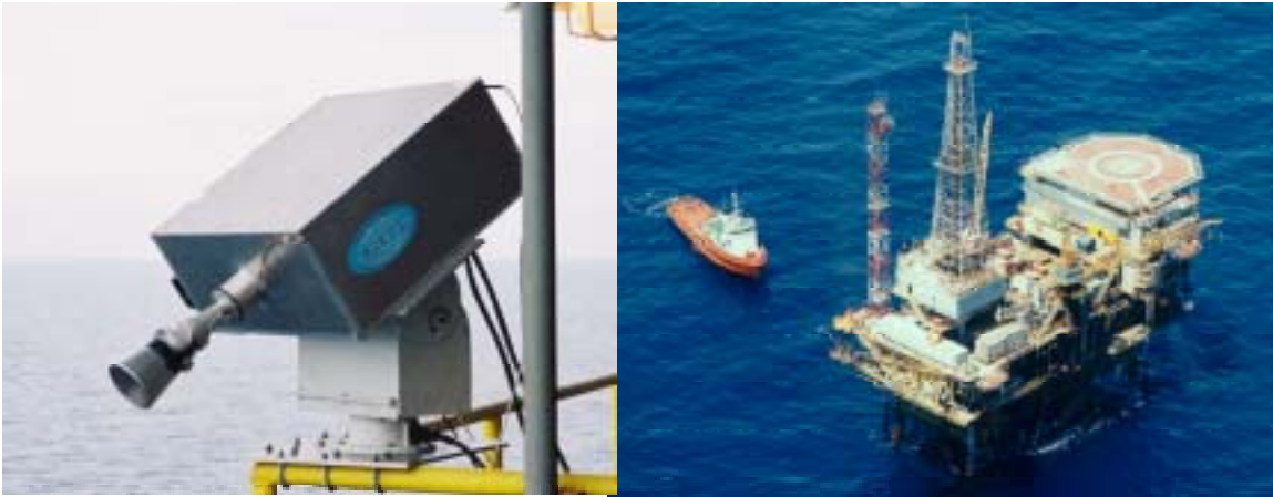
Figure 1. The UMass Ka-band polarimetric radiometer (left) on the Casablanca oil platform (right) in the Mediterranean Sea during the Wind and Salinity Experiment 2000.
