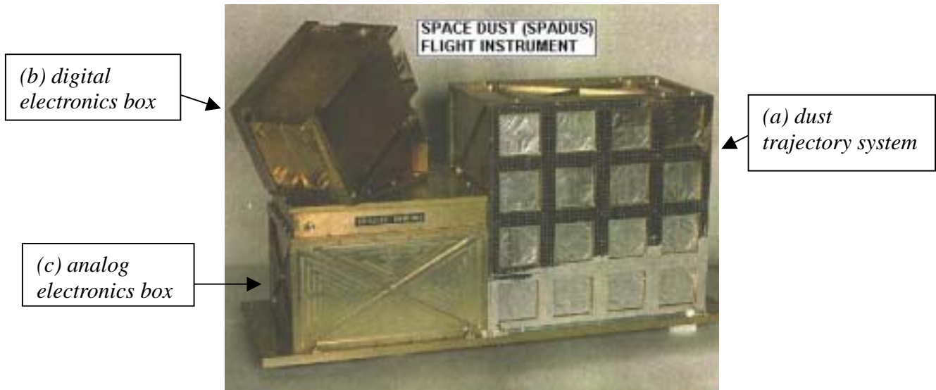
Figure 1: Photograph of the SPADUS Flight Instrument showing the dust trajectory system, the digital electronics box, and the analog electronics box.
